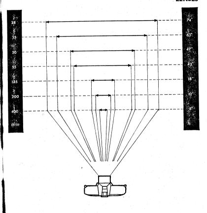
Lenses available for the Mamiya Sekor cover the range of focal lengths from 28 mm. to 400 mm. with angles of view from 74° to 6°. The arrowed lines above compare the angles of view (right) for each focal length (left).
