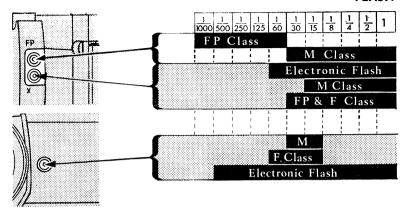
All models except the 528 TL have FP and X flash contacts for synchronisation of bulbs and electronic flash. The shutter speeds and settings that can be used are shown diagrammatically above. The 528 TL contacts are both of the X type for electronic flash at all speeds and bulbs only at the slower speeds.
