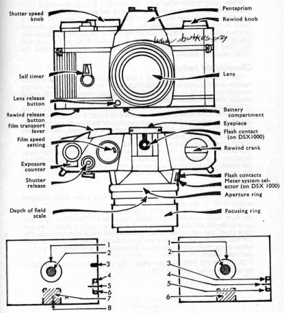
Left: DSX1000 finder. 1, Clear ground glass. 2, Microprism. 3, Low-light warning. 4, Over-exposure zone. 5, Meter needle. 6, Under-exposure zone. 7, Spot metering area. 8, Meter system indicator. Right: MSX500 finder. 1, Clear ground glass. 2, Microprism. 3, Over-exposure zone. 4, Meter needle. 5. Under-exposure zone. 6, Spot metering area.
