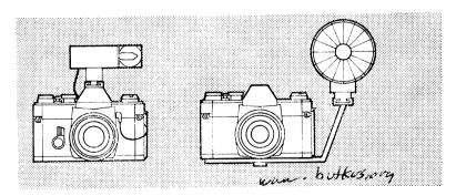
The flash gun can be connected to the camera with the aid of an accessory shoe fitting (left) or with the id of a flash bracket (right). The latter is generally preferable so that the flash is not dead in line with the lens.
