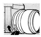
The Mamiya Sekor cameras are fitted with a manual-auto lever on the lens mount. The diaphragm closes down to the pre-set aperture when the lever is moved to M so that the effect of the shooting aperture on depth of field can be seen on the focusing screen.
