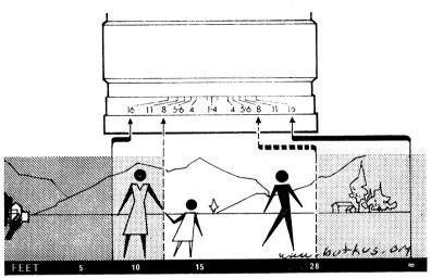
Mamiya Sekor lenses have a depth of field scale engraved on the lens barrel behind the focusing ring. It has lines pointing to the distance scale from a set of aperture numbers each side of the focusing mark. Each pair of lines from the same aperture number indicates the nearest and farthest planes of sharp focus at that aperture. Thus, with a standard lens set to 15 ft., the depth of field extends from  $8\frac{1}{2}$  ft. to infinity at f 16 or, at f 8, from 12 ft. to 28 ft.
