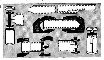
To load standard 35 mm. cassettes, trim the required length of film at each end or use ready-trimmed refills. Push end of film into cassette spool or attach with adhesive tape. Handling the film by its edges only wind it on to the spool and insert spool in cassette, allowing an inch or two of leader to protrude. Replace cassette cap.
