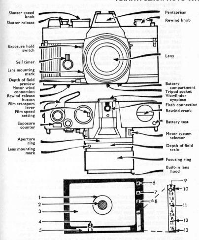
Mamiya Sekor Auto XTL Finder: 1, Clear ground glass. 2, Microprism. 3, Fresnel screen. 4, Shutter speed indicator. 5, Shutter speed scale. 6, Manual indicator. 7, Average metering indicator. 8, Spot metering indicator. 9, Stopped-down metering index. 10, Under-exposure zone. 11, Aperture scale. 12, Meter needle. 13, Over-exposure zone.
