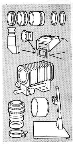
The wide range of accessories for the Mamiya Sekor cameras includes (from top to bottom) extension tubes and close-up lenses angular viewfinder, rubber eyecup, eyepiece correction attachment, extension bellows, microscope attachment, lens hoods, and copying stand.
